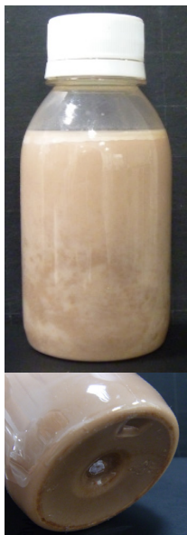
Creaming and slight cocoa sedimentation
