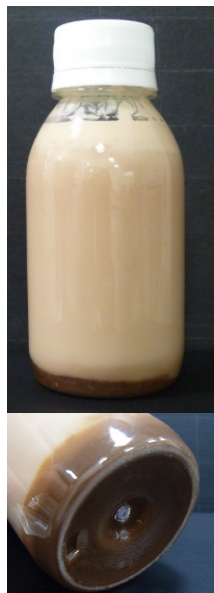
Heavy creaming and cocoa sedimentation
