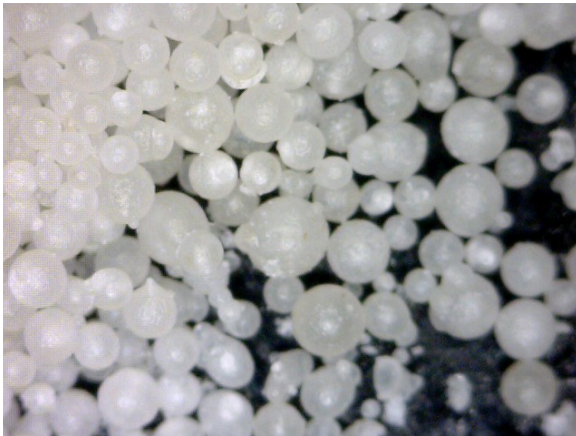
Stabilisers are encapsulated by emulsifiers. Product is in bead form. Particle size is generally larger compared to typical emulsifiers.
